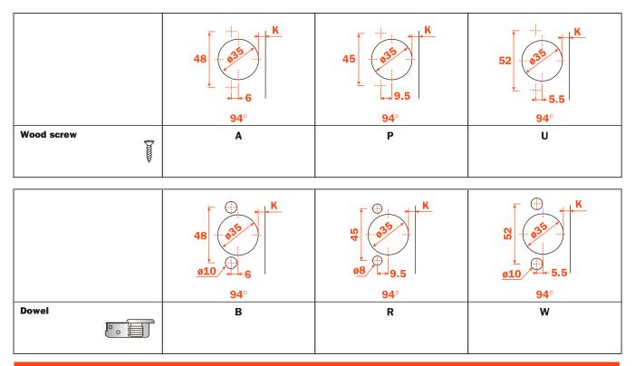
Use this table to identify the available drillings and fixings. Fill the third position of the hinge code number with the letter or the number corresponding to your choice. I.e.: C3\_BAE9.
