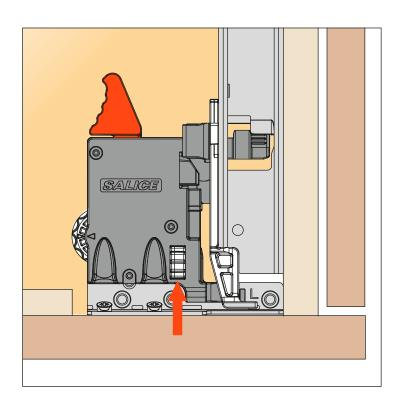
For sideways adjustment, it is recommended that the adjusters on the clips are operated in the same direction, in order to maintain the correct alignment and movement of the runners.
