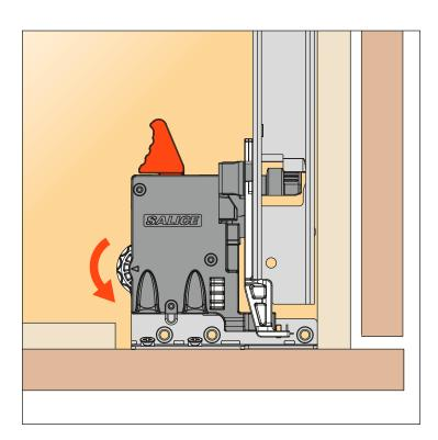
Rotate the white wheel towards the inside of the drawer to reduce the gap between the frontal and the side. This operation is tool free.
