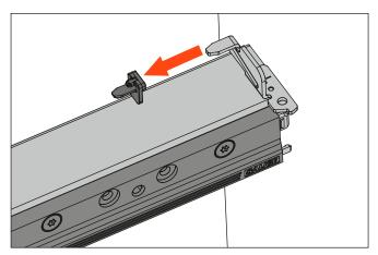
Insert the lever for the tilt adjustment, both right and left
