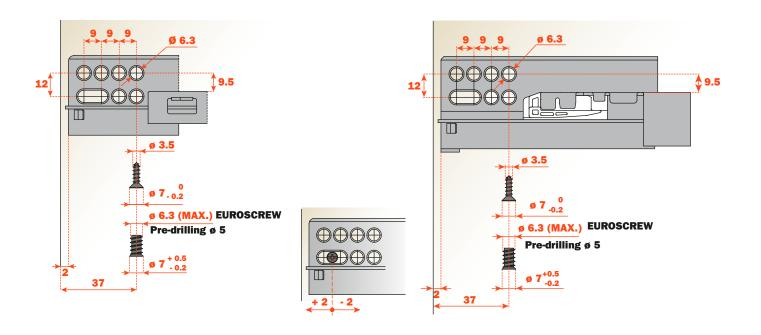
The oval slot allows the easy alignment of drawer frontals particularly in multi drawer and Push applications.
