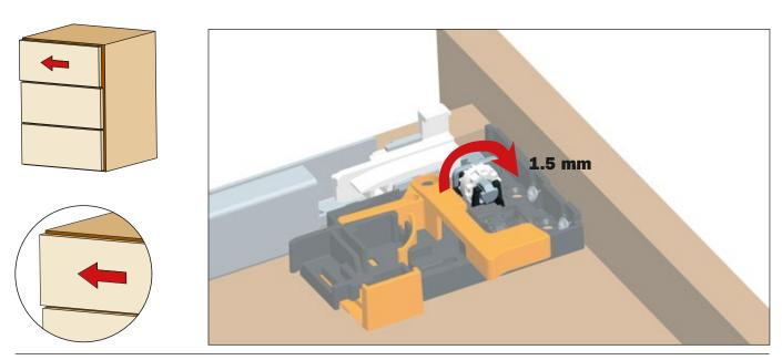
Rotate the white wheels towards the back of the drawer to adjust right.
