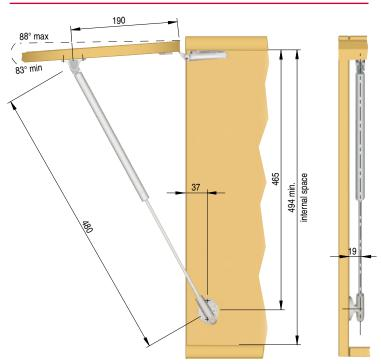
The dimensions of the above drilling plan refer to carcases which use standard sprung hinges and mounting plates 0mm.
