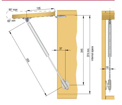
The dimensions of the above drilling plan refer to carcases which use standard sprung hinges and mounting plates 0mm.
