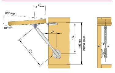
The dimensions of the above drilling plan refer to carcases which use standard sprung hinges and mounting plates 0mm.
