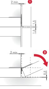
A 0,5 mm gap between the door and the platform laying underneath doesn't interfere with the opening.
