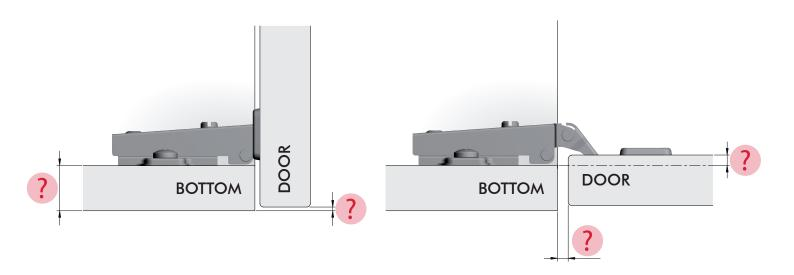
Note: standard hinges to be used must be unsprung.
