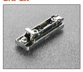
Die-cast mounting plates. Fixing: Euroscrew. Drilling ø5x11.
