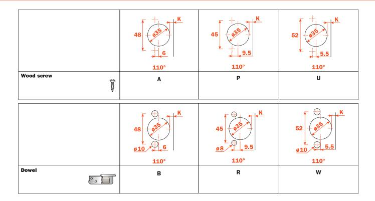
Use this table to identify the available drillings and fixings. Fill the third position of the hinge code number with the letter or the number corresponding to your choice. I.e.: CB\_2A99.
